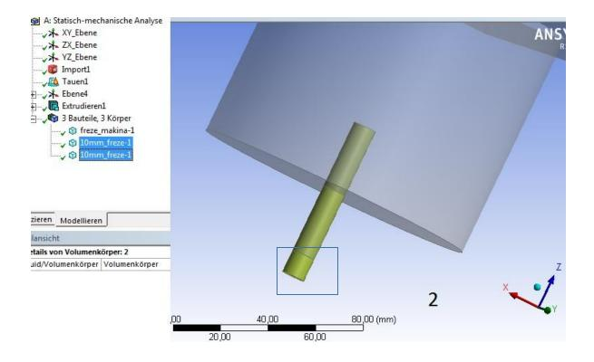
İ cut the "end mill" in 2 parts in order to analyse only the first 10mm
