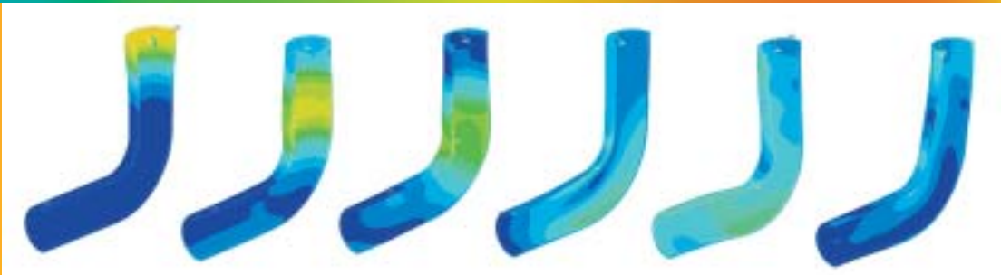
Figure 4. In this FSI analysis of blood flowing in an elastic artery, the fluid pulse travels from top to bottom of the artery, deforming the structure as it passes through.
