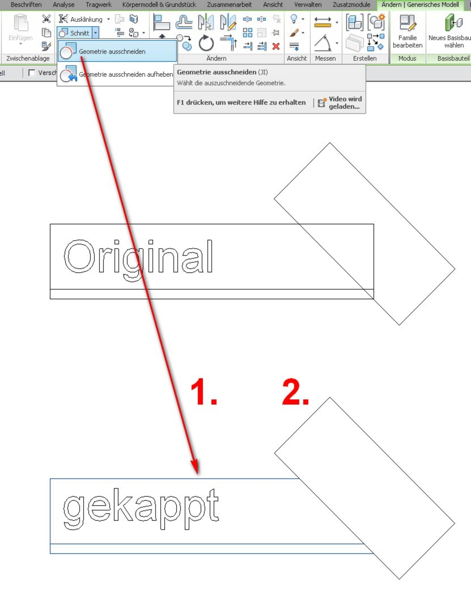
Software interface showing various toolbars and menus. The 'Schnitt' (Cut) menu is active, with 'Geometrie ausschneiden' (Cut Geometry) selected. Other visible options include 'Ändern' (Change), 'Ansicht' (View), 'Messen' (Measure), 'Erstellen' (Create), 'Modus' (Mode), and 'Basisbauteil' (Basic Part).
