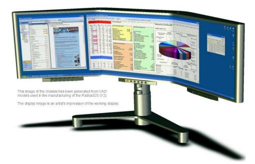
The Radius 320<sup>™</sup> incorporates three 20.1" LCD panels into a continuous display system with a total of 5.8M pixels. With the individual panels wrapping around the user, and height and tilt adjustment, the Radius 320™ provides an ergonomically-friendly viewing experience across a 50-inch diagonal.
