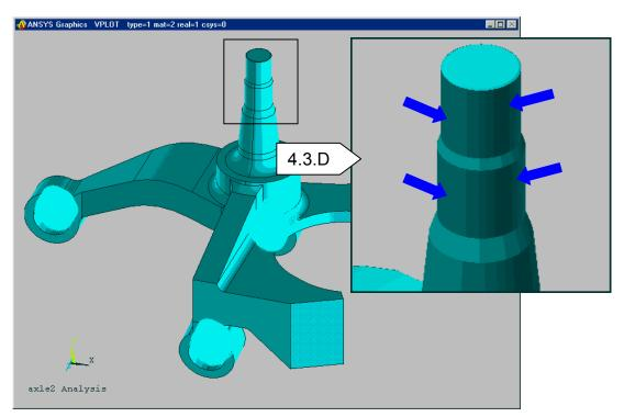
G. Input **-2780** newtons for the Force along the X-axis and **8230** newtons for the Force along the Z-axis.
