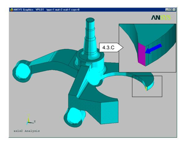
D. Input **600** newtons for the **force along the Y-axis** and **-1450** newtons for the **Force along the Z-axis**. Click on **OK**. The symbols for the force will appear on the small area.
