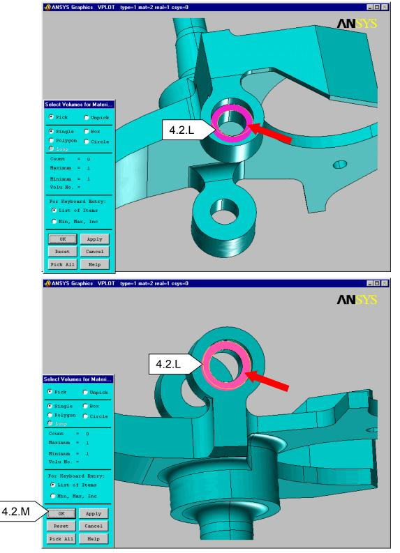
L. Pick the bottom face of the counterbored hole on both the upper and lower attachment locations as shown. (Just the 2 holes shown)
