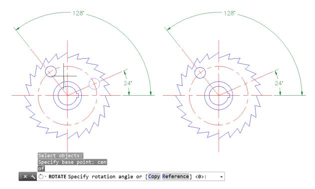
In the second scenario, you need to create a copy the circle and rotate it to new position at 128 degrees. But we do not know the current angle. How would you do this? Do you use the **Copy** subcommand? Do you use the **Reference** subcommand? And at what angle do you rotate to?
