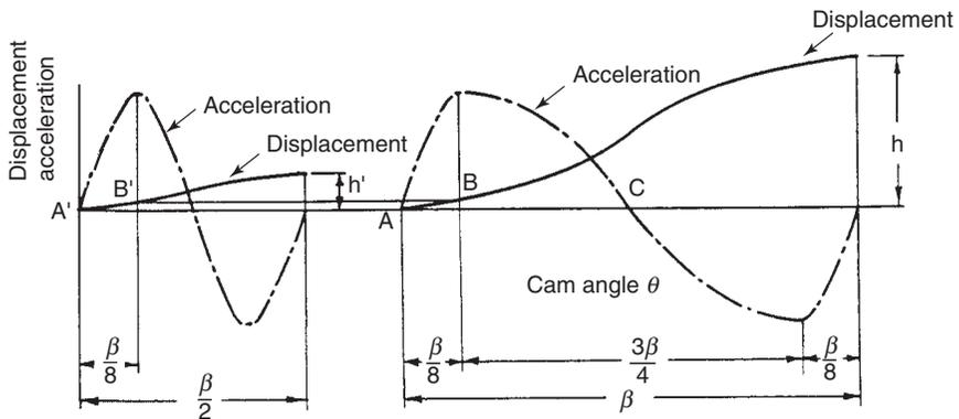
(a) Cycloidal curve. (b) Modified sine curve.
