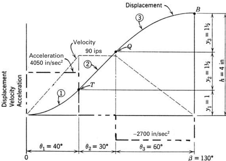
FIGURE 3.3. Example modified constant velocity curve.
