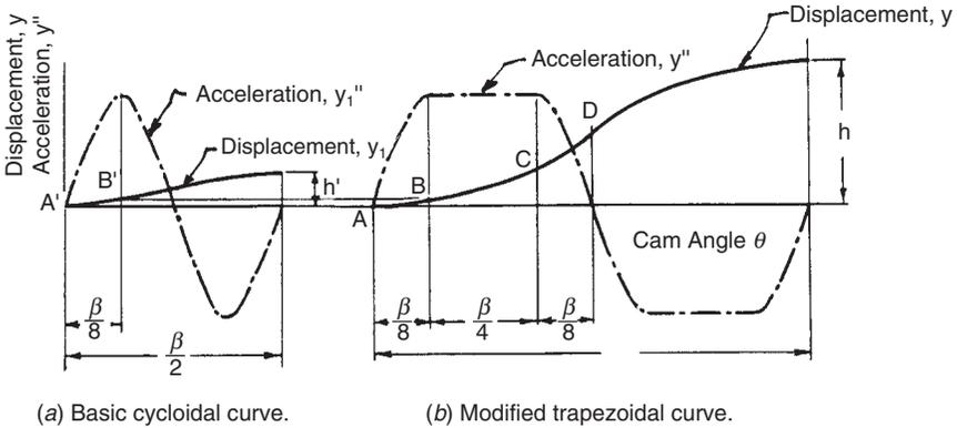
FIGURE 3.5. Modified trapezoidal acceleration curve.
