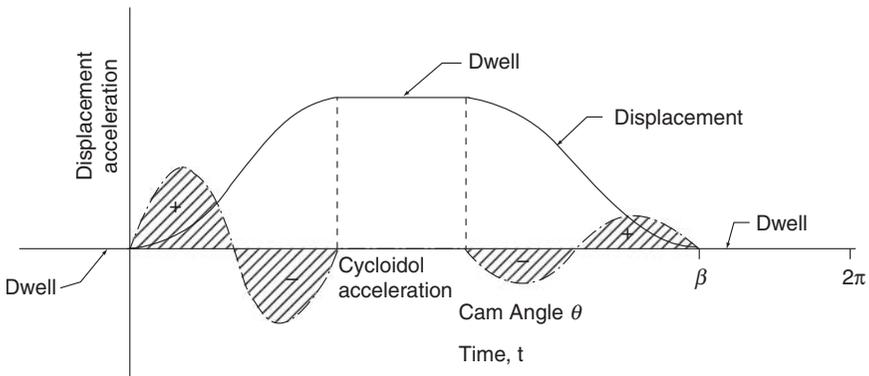
FIGURE 3.1. Dwell-rise-dwell-return-dwell cam with cycloidal acceleration curves.
