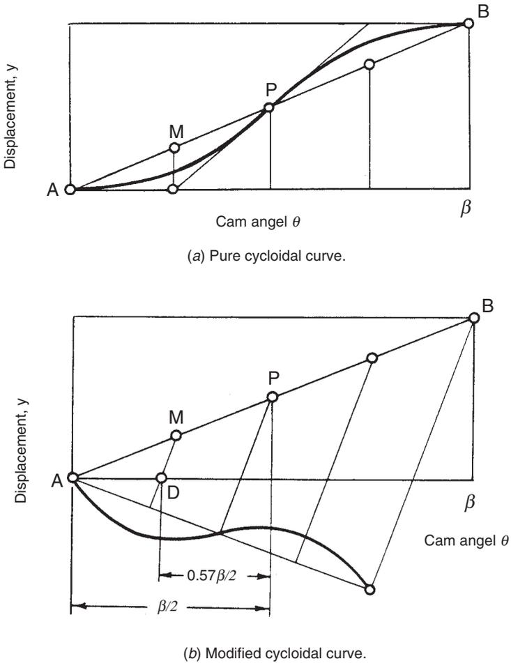
FIGURE 3.12. Modified cycloidal curve construction.
