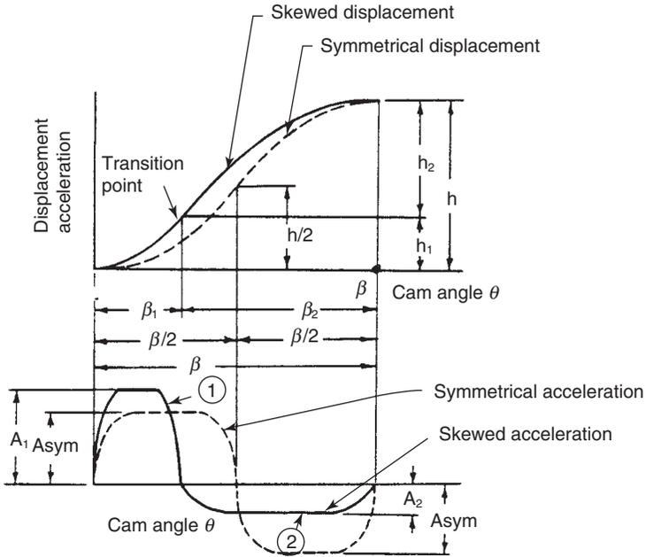
FIGURE 3.7. Skewed modified trapezoidal curve.
