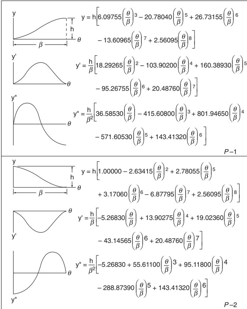
FIGURE 3.17. Eighth-degree polynomial motion characteristics.
