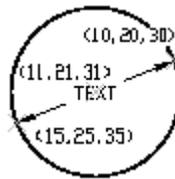
The point (15,25,35) specifies the first point of the dimension line on the circle/arc and the point (10,20,30) specifies the center of the circle/arc. The point (11,21,31) specifies the midpoint of the dimension text.
