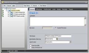
10. Linking 1.1SubAssembly to 1.1SubAssembly-Bob project for Assembly level authorization: Drag and drop 1.1SubAssembly-Bob into 1.1SubAssembly-Bob project by holding CTRL key and answer dialog box with Yes.
