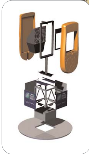
The Nokia Design explosive view & construction.
