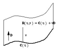
• C must not be an intersection curve or a trimmed curve.
