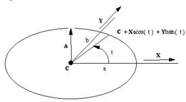
• Y and b are the minor axis and minor radius respectively.
