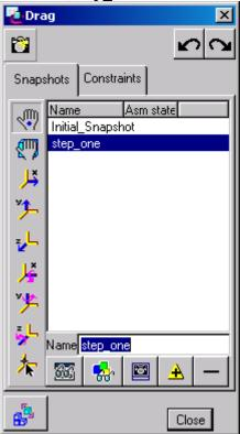
Lets start to move a component, select Translate in X icon, Pick on the Knob\_Spring component and move it to the right, away from the assemble. When you get it to be were you want it, click the first mouse button (FBM).
