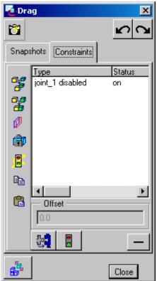
Select the Enable/Disable Constraint icon, This will allow you to select a constraint, select the following pin-joint:
